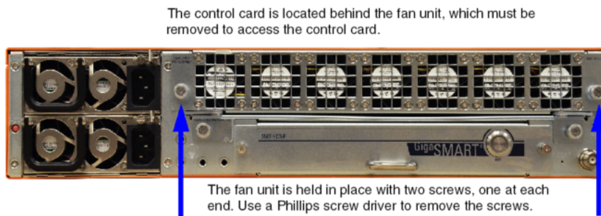
Figure 1 Replacing a Control Card
